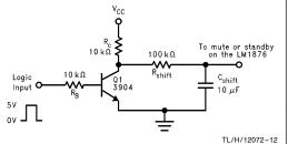
FIGURE 5. Level Shift Circuit
