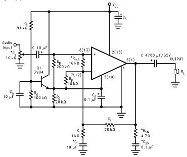
FIGURE 3. Single Supply Amplifier Application Circuit
