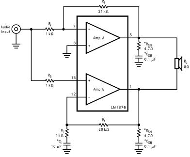
FIGURE 2. Bridged Amplifier Application Circuit
